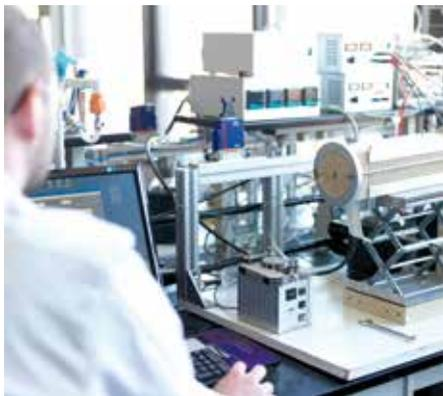
An electrolysis cell uses electricity to split water molecules ( $H_2O$ ) into hydrogen ( $H_2$ ) and oxygen ( $O_2$ ). In this way, electrical energy is transformed into chemically bound energy in the hydrogen molecules. This is the reverse of the process that occurs in a fuel cell.
