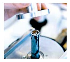
Magnetic refrigeration is an emerging technology that uses solid, non-volatile magnetic materials as the active components and water or alcohol as the medium for heat transport. The technology has great potential for low energy consumption and environmentally friendly cooling at a competitive price.
