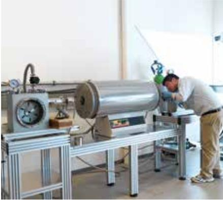
The electrical resistance of a superconductor vanishes when it is cooled down below its critical temperature. This feature makes superconductors interesting for many applications, including power cables and high field magnets. Cables made of classical materials such as copper suffer not only from power dissipation and heat losses, but also from a significantly lower current density. As a consequence, much larger currents can be transferred in superconducting wires with a comparable diameter.
