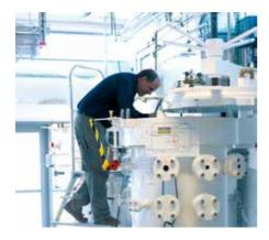
An electrolysis cell uses electricity to split, e.g., water molecules ( $H_2O$ ) into hydrogen ( $H_2$ ) and oxygen ( $O_2$ ). In this way, electrical energy is transformed into chemically bound energy in the hydrogen molecules. This is the reverse of the process that occurs in a fuel cell.
